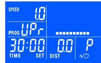
Use ↑/↓ buttons to program speed and incline for each segment, press ENTER to confirm.
