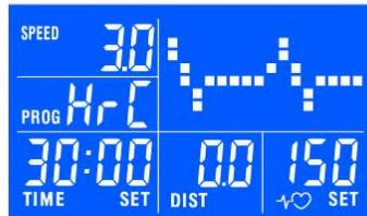
Use ↑/↓ buttons to program target heart rate, press ENTER to confirm
