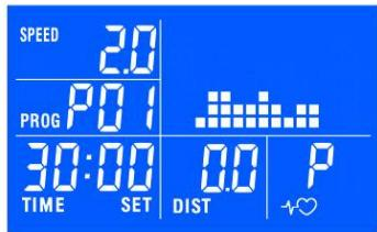
Press ENTER to set time, use ↑/↓ buttons to adjust values, press ENTER to confirm.
